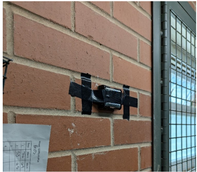
Figure 5: Audiomoth taped to wall.
