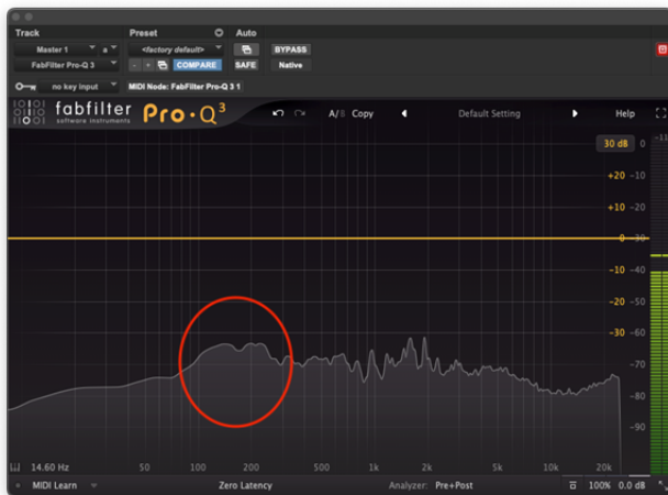
Figure 9: Screenshot from Fabfilter Pro-Q 3 demonstrating background noise level.
