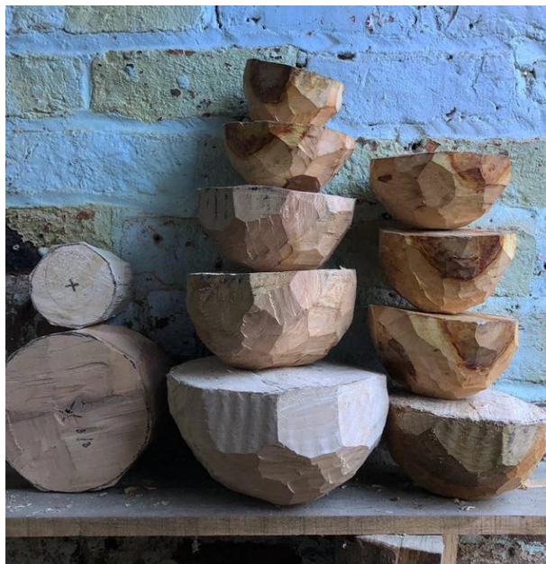
Figure Four: The Variety of Sizes and Shapes of Roughed Out Blanks (© Skapa Woodturning)
