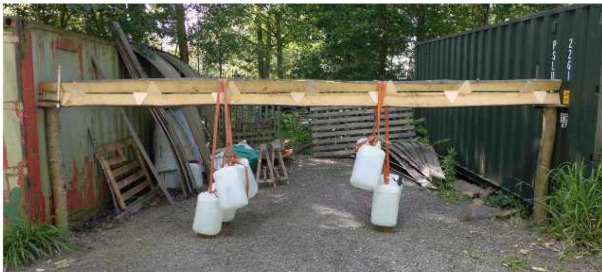
Figure 8. Load test in progress with 240kg of load distributed between x2 load points along the 6000mm XR Beam.
