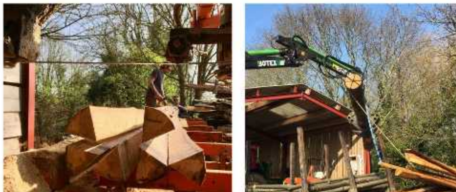
Figure 2a/b. Radial cutting of roundwood log on a mobile saw mill.
