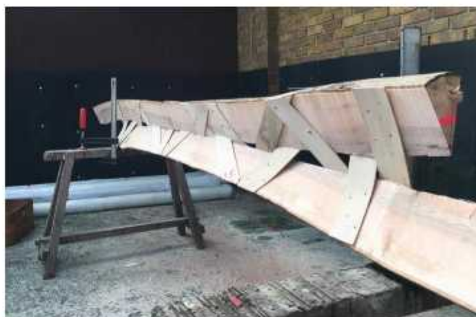
Figure 5. 1 st prototype made from Ash ( Fraxinus Excelsior ) radially cut in 1/8 th segments and connected with 3-ply 3mm x 70mm Ash plywood.
