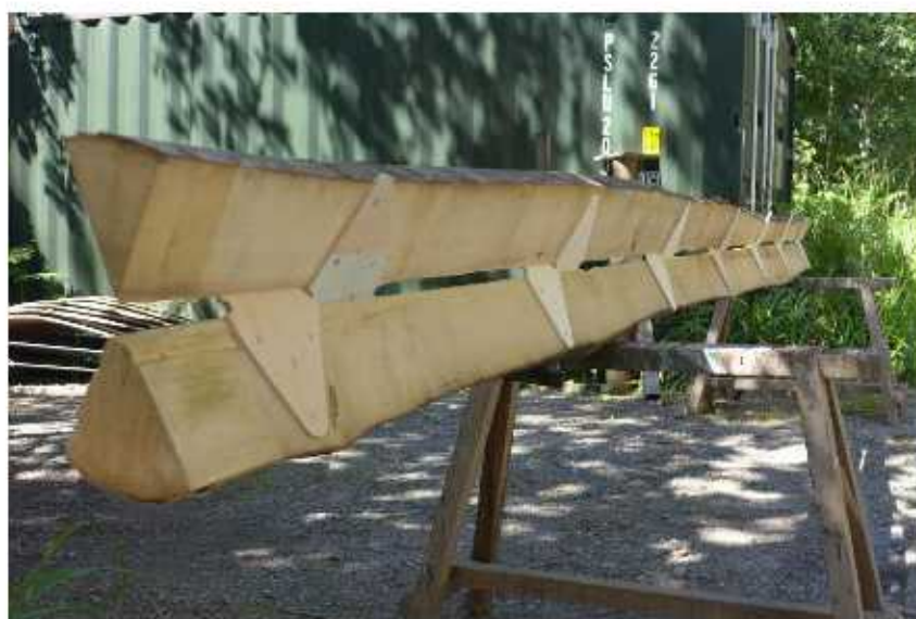
Figure 6. The 2 nd prototype made from Sweet Chestnut ( Castanea Sativa ) with birch plywood gussets
