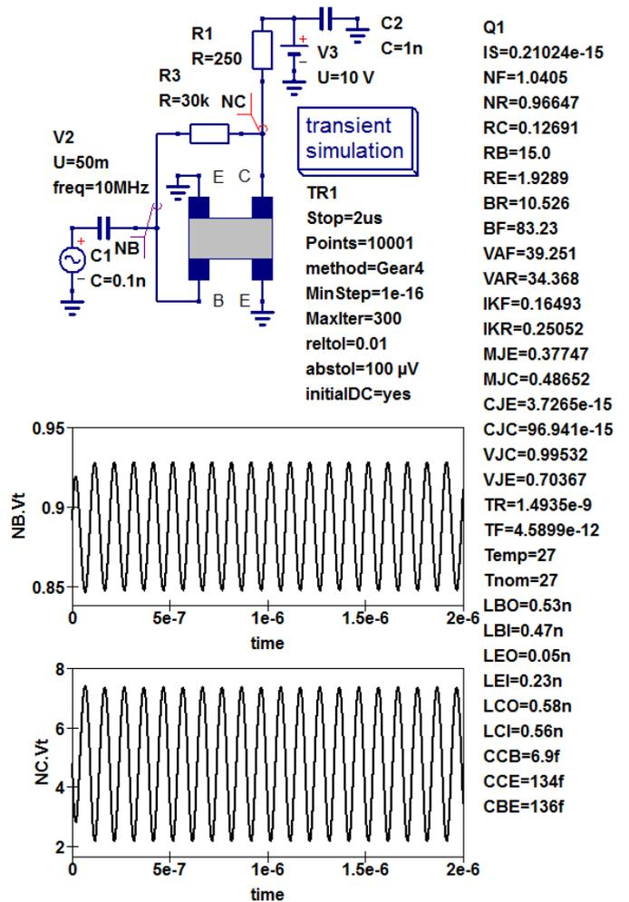
Figure 7. A class A npn BJT RF amplifier with collector feedback: transient simulation test circuit with directly coupled voltage test probes NB and NC and time response output waveforms for a sinusoidal input signal of 50mV peak, 10MHz frequency and zero input phase.
