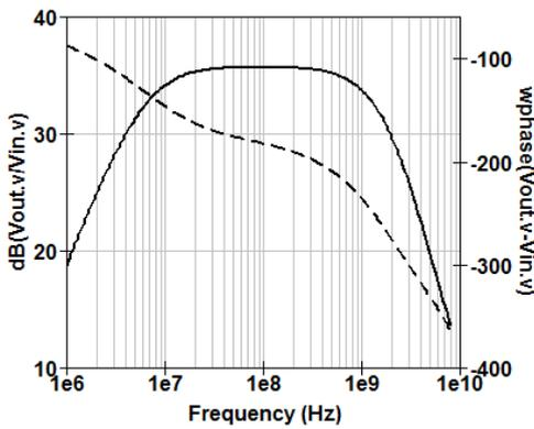
Figure 4. A class A npn BJT RF amplifier with collector feedback: small signal AC test circuit and example gain and phase response curves; legend: solid line =  $\text{dB}(V_{\text{out.v}}/V_{\text{in.v}})$  the amplifier gain in dB and dotted line =  $\text{wphase}(V_{\text{out.v}}/V_{\text{in.v}})$  the unwrapped phase of the amplifier gain in degrees.
