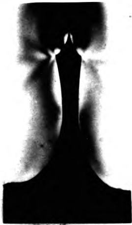
Fig 96. Photograph of d.c. sample pintip showing stress distribution around tip. (d.c. sample 3 x10mag.)
