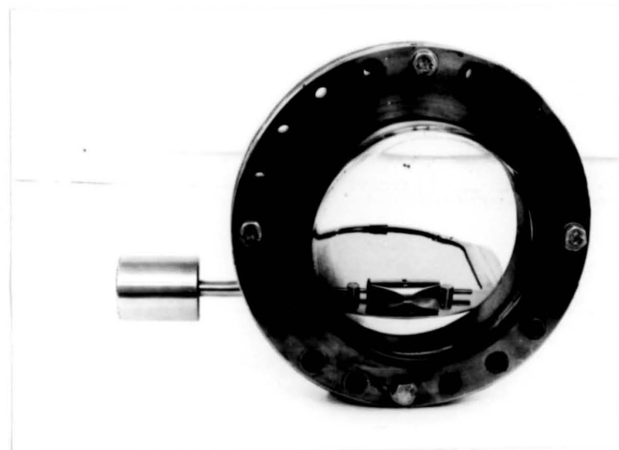
Figure 2.11 Counterbalanced viewport shutter.
