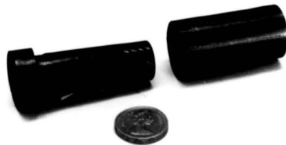
Figure 2.19 Cracked silicon source cell after heating to > 1500^{\circ}\text{C} .
