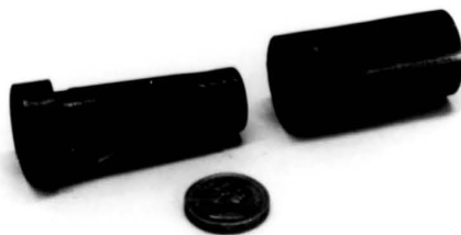
Figure 2.19 Cracked silicon source cell after heating to > 1300^{\circ}\text{C} .
