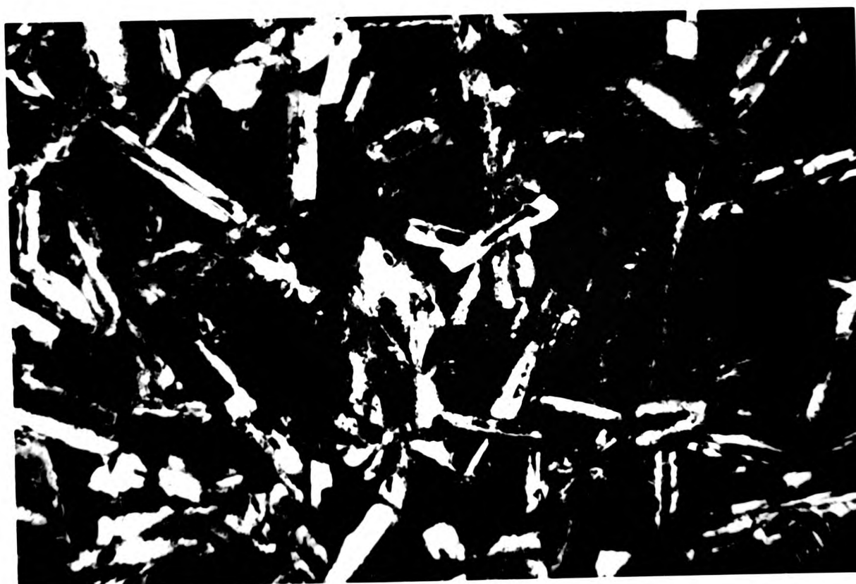
Plate 4.20 Skeletal feldspars containing glass inclusions, the matrix consists of chlorite, magnetite and pyroxene all of which have been thermally metamorphosed. Inner Centre Two, Lighthouse. (x4, xpl)
