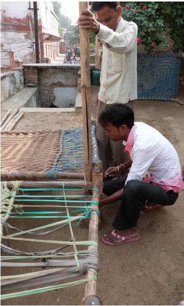
Creating the bamboo structures with charpoy beds
