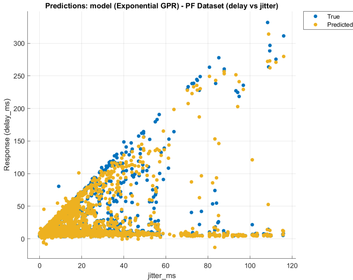
Figure 5.3: EGPR model performance for delay versus jitter under PF scheduling. Delay generally increases with jitter, confirming a positive association; however, the wide scatter – especially at low jitter – shows substantial variability that the model does not fully capture.
