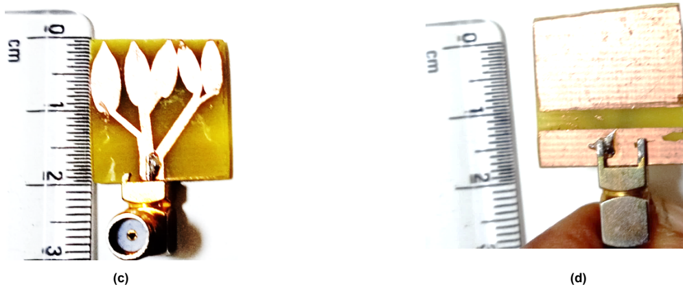
Figure 2. Geometry of sneezewort plant inspired antenna (a) Top Structure (b) Bottom Structure (c) Top of Fabricated antenna (b) Bottom of Fabricated antenna
