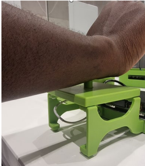
Figure 6.11: Biosensor testing setup showing the user's forearm placed over the patch platform to evaluate electromagnetic interaction with the skin.
