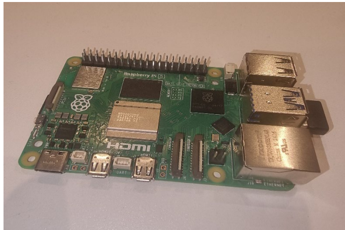
Figure 6.14: Raspberry Pi 5 Model single-board computer featuring a quad-core processor, dual HDMI outputs, USB 3.0 ports, and GPIO header.
