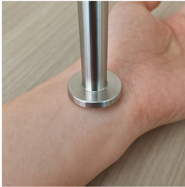
Figure 4.7: DAK probe on the human subject's wrist.
