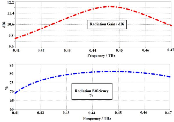
Fig.3. 2-D gain and efficiency plots versus frequency.
