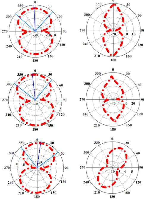
Fig.4. E- and H-planes radiation patterns of the proposed structure at the operating frequencies of 410, 450, and 470 GHz.
