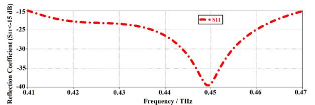
Fig.2. Reflection coefficient ( $S_{11} < -15 \text{ dB}$ ) of the proposed metasurface on-chip antenna.
