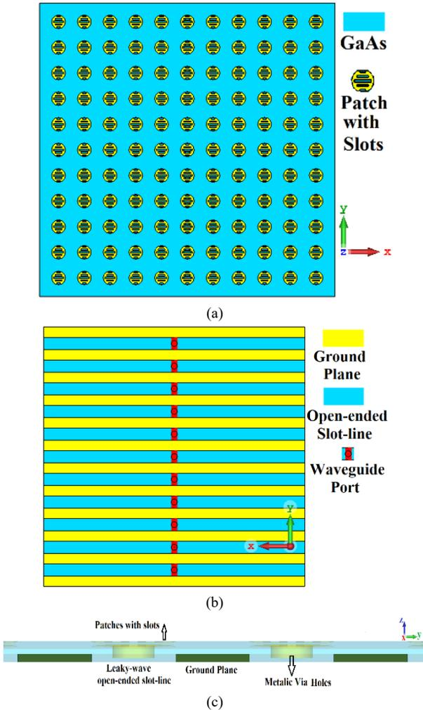
Fig.1. Layout of the metasurface on-chip antenna.
